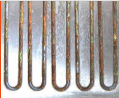
uncoated channels after a salt spray test with a duration of 230 hours (NaCl solution acc. to DIN EN ISO 9227) with massive corrosion.
