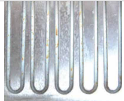
coated channels after a salt spray test with a duration of 230 hours with minimum corrosion.
