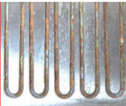
Uncoated channels after 230 hours of salt spray testing (NaCl solution as per DIN EN ISO 9227) with heavy corrosion
