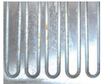
Coated channels after 230 hours of salt spray testing with minimal corrosion
